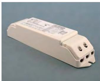
LLVC12A Driver 100V~240V, 11W Máx: 12x 1W (350mA) dim.: 162 x 40 x 30 mm
