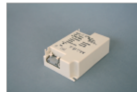
LTVC18A Driver 100 V~240 V, 16 W Máx: 18x1 W (350mA) Dim: 102x62x30mm
